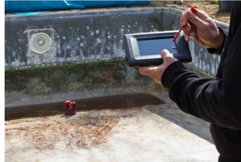
Measure a height reference, e. g. the floor drain as zero-level
